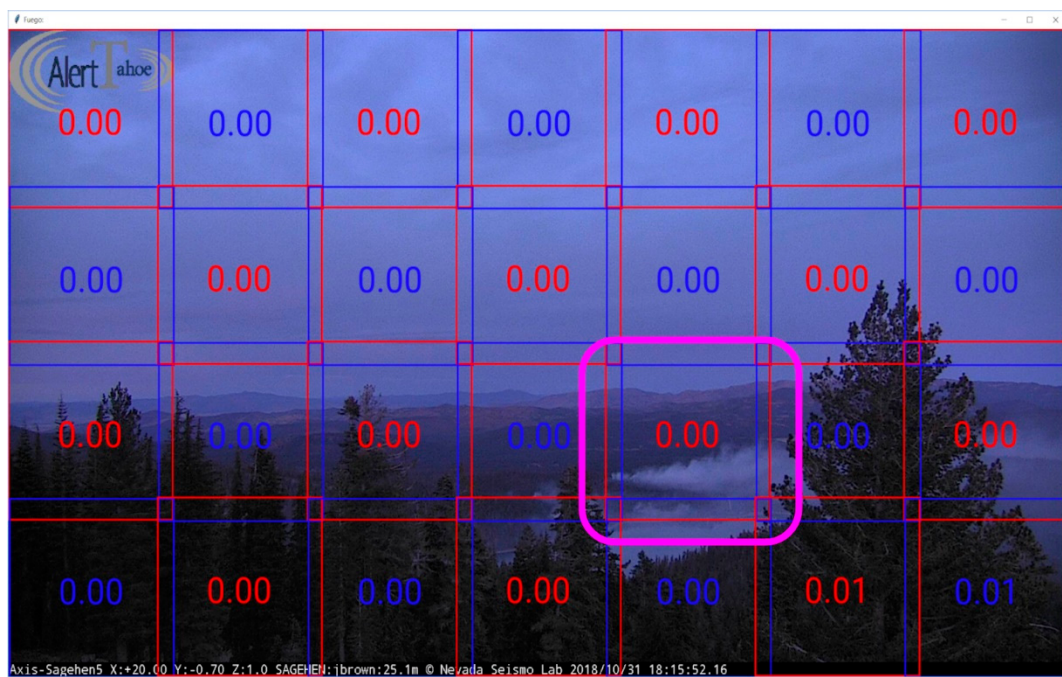
Figure 5. False negative, where smoke in highlighted segment is not detected. Our hypothesis is that this event resembles fog.
