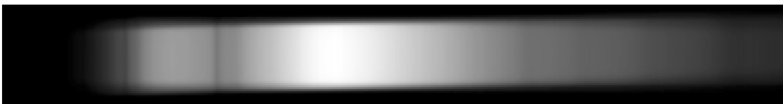
Vertically stretched 4 second spectra of Gamma Geminoris. The diffraction grating allows spectroscopy at approximately R500.
